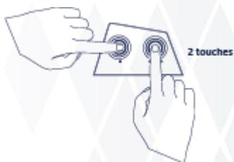
Click simultaneously the "FAN SPEED" and "ON / OFF" buttons two times quickly.
