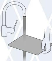
Wash the filter under running water. Make sure that the filter is completely dry before reinstallation.
